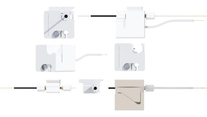
SIMPLE LINK UNO 1/32 incorporates a VICI Cheminert 360 nano volume fittings, with a 1/32" sleeve on the column side and a 360  $\mu m$  ferrule on the emitter side. Inner diameter 50  $\mu m$ , estimated swept volume ~1nL
