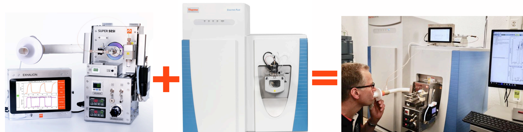
Figure 2. breath analysis system, comprising the breath guiding system, the SESI ionizer, and the MS
