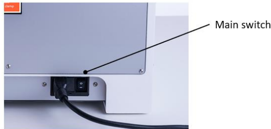
Figure 3. DESAMPLER, main switch
