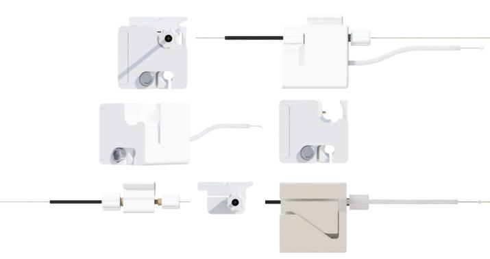
SIMPLE LINK UNO 1/32 incorporates a VICI Cheminert 360 nano volume fittings, with a 1/32" sleeve on the column side and a 360  $\mu$ m ferrule on the emitter side. Inner diameter 50  $\mu$ m, estimated swept volume ~1nL
