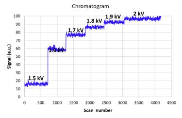
The optimum voltage required by the LOTUS emitters will be slightly lower than the classic. To adjust the voltage, start with a rather low voltage (i.e. 1.5kV) and rise it by 0.1kV increments, until you get a nice and stable signal, and signal increases are not significant.
