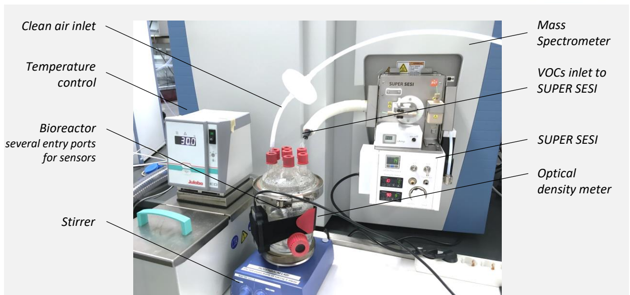
Figure 1: experimental setup assembled at the Prof. Blanks lab at the Institute of Applied Microbiology (iAMB) of the RWTH Aachen University ( https://www.iamb.rwth-aachen.de ). Clean air is passed through an active charcoal filter before it is introduced in the bioreactor. The reactor temperature is set at 30° C. VOCs released by the medium and the cell metabolism are passed through a ceramic filter to eliminate aerosols and carried by the air flow into the Super SESI. Optical Density, and VOC signals are used to understand the different stages of cell culture growth.
