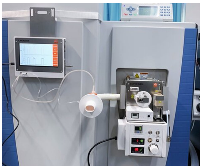
Figure 3. Instrumentation for Breath analysis by SESI-MS. The Exhalation interface connected to a Super SESI, and coupled to an Q-Extractive mass analyzer.
